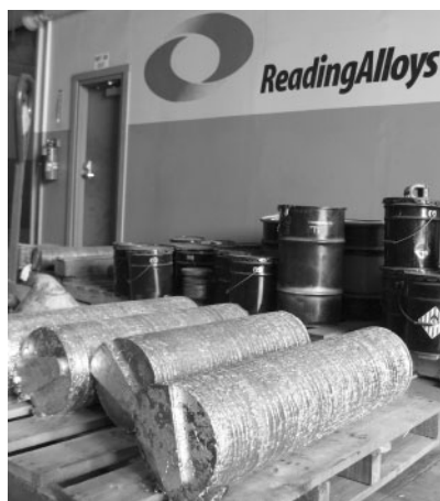
1 High purity electron beam (EB) melted ingots, each weighing approximately 385 kg (850 lb)
