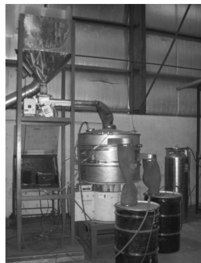
3 Typical three-deck screener used in production of titanium powders
